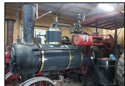
(Above) Aaron's latest project is making a jacket for the Advance. The pieces of wood act as insulation. After the sheet metal is cut and fitted it was painted a dark gray. (Below) The brass bands keep it in place.
