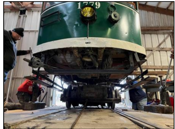
The trucks were removed from the 1779 car so that they can be repaired by the Gomaco Trolley Company in Ida Grove, IA.
