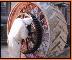
Gregg Crew removes years of grease and grime from the gear of a back wheel.
